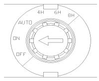
Fig4 (Rotary Time Control Switch)
